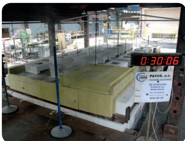
Fig. 11 Sample after 30 minutes – fire protection system Isover FireProtect® fulfils its function for 100 %, roof is without any deformation (bending stress, the same as would be under cold conditions)
