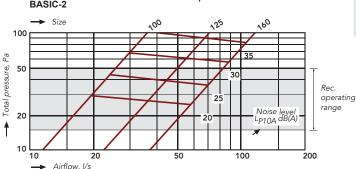
**Note** Air flow in the duct outlet must not exceed the speed in any of the distribution ducts. The top edge of the distribution duct must always be below the bottom edge of the connection duct. The revised values are based on measurements with a straight section corresponding to 4 diameters after BASIC has been calculated from the edge of the inlet. A shorter straight section may cause noise and pressure problems.
