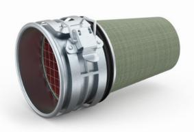
BASIC 2 non-return dampers prevent fire gases from spreading through the supply air system in supply/exhaust ventilation systems with fans in operation during fire. Suitable for apartments, hotels, hospitals and retirement housing. Type approved.
